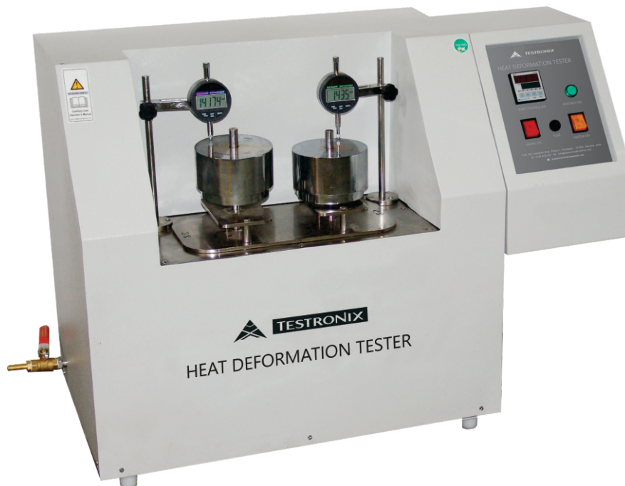
Dial gauge with Indenter tip to measure deflection
