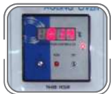
PID Temperature Controller
