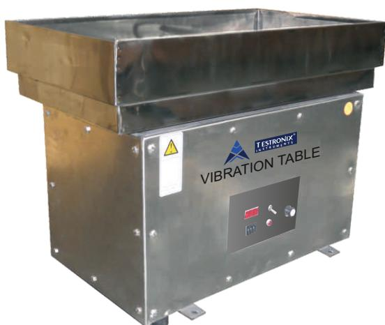
Vibration Table is a consistent tool useful to simulate the carbon dioxide present in test specimen through automated, motorized shaking of bottle specimen. Accurate and reliable testing equipment in PET Bottles industry.
