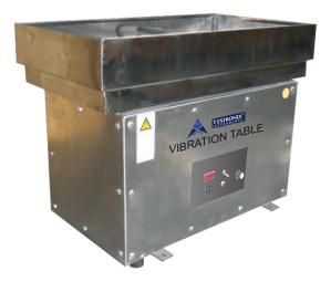
Vibration Table is a consistent tool useful to simulate the carbon dioxide present in test specimen through automated, motorized shaking of bottle specimen. Accurate and reliable testing equipment in PET Bottles industry.
