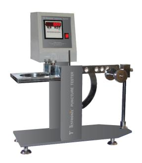
**Puncture Resistance Tester** is a consistent tool useful to determine the resistance to puncture of paper and paper board. Puncture Resistance Tester is used to measure the resistance of paper, paper board and other similar materials when subjected to puncture and determination of absorbed energy. Puncture Resistance Tester is designed as per standards TAPPI –T803, ISO 3036 and ASTM D781.
