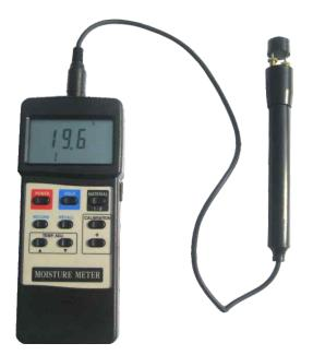
Moisture Meter is the latest high sensitivity hand held moisture meter developed specially for the packaging industry. The portable moisture meter is used for measuring the moisture content of paper, corrugated sheets, cardboard stocks, kraft paper, paper tubes & paper bales,quickly and effectively.
