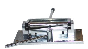
**Conical Bending Mandrel** is a laboratory apparatus to bend coated test panels over a conical shaped mandrel in order to assess the elasticity or resistance of a coating paint or varnish to cracking; elongation and / or detachment from a metal test panel in accordance with ISO 6860 and ASTM D522.
