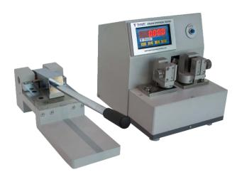
Crease Stiffness Tester is a multi-function stiffness tester, mainly used for measuring cardboard, color box (such as cigarette case cosmetic box) of the indentation force (that is, 90 crease of the rebound force), can also measure a variety of cardboard Bending stiffness is achieved on the same instrument with two measurements: 15° flexing Degrees and 90° crease stiffness.
