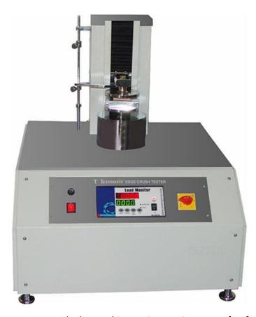
Vertical Paper Core Tester reveals the crushing resistance in terms of Kgf unit
