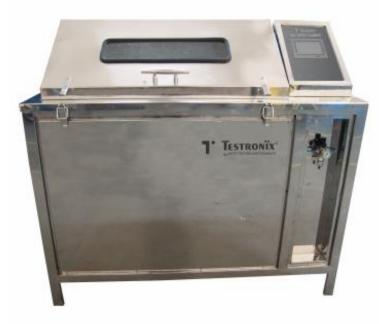
Salt Spray chamber SS (HMI- Touch Screen) is one the most accurate instruments for measuring the corrosion resistance of coating when exposed to highly corrosive environment. In industries the material is exposed to various types of climatic conditions and chemical fumes which cause corrosion of components and parts. Hence a salt spray chamber plays a pivotal role to test the specimen and analyse the quality of material being used by manufacturers.
