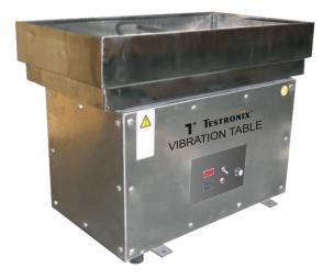
The Vibration Table is an accurate and affordable solution for calculating the damage caused by repetitive movement caused to materials/ boxes during transportation. The durability of the packaging must be checked beforehand so as to provide the best quality to
