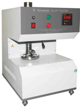
Scuff Resistance Tester is a very accurate instrument to evaluate the rub resistance between two stickers or any general printed material. The term scuff implies the rubbing of two materials against each other.
