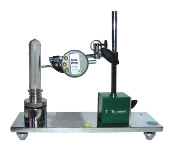
Preform Perpendicularity Tester is a consistent tool that helps the manufacturer in testing the perpendicularity of PET preforms. It is based on the principle to test the accuracy of the shape and size of preforms.
