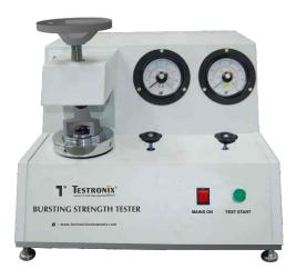
Bursting Strength Tester Analogue is a consistent tool to indicate the Strength and performance of material like Rexene, leather, paper boards, paper, uneven boards and boxes, industrial fabric and solid fiber boards, filter cloth, plastic films, Foils, sheets, etc. Bursting Strength Tester is manufactured under various Test Standards ASTM D 3786–01, ASTM D 3786 – 80A, ISO 1060 PART-1 1987.
