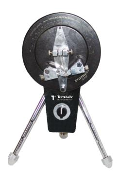
**Stiffness Tester** is a consistent tool useful to measure stiffness or flexural rigidity of paper and paper board. Stiffness Tester is used to determine the resistance of paper and paper board to bending. The economic value of paperboard highly depends upon its bending resistance or stiffness.
