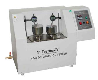
**Heat Deformation – HDT/VSP Tester** is a consistent tool useful for determining the ability of a given polymer to bear load at elevated temperatures. Accurate and reliable deflection or deformation is important component in plastics industry. Heat Deformation HDT/VSP Tester is designed as per standards IS 2530-1963, ISO 75-1(2004)-E, ASTM D648-01, ASTM D1525-00.
