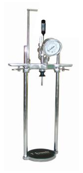
Carbonation Assembly is a consistent tool useful for determining the pressure and temperature of carbonated drinks. Accurate and reliable testing assembly in PET Bottles industry.
