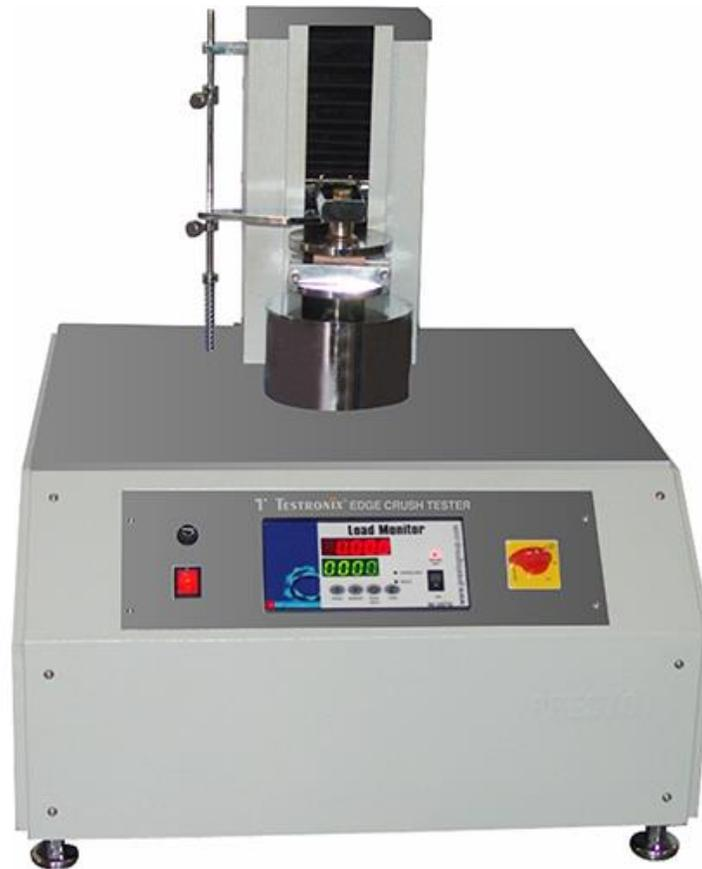
*The peak load is measured in the unit of pounds per lineal inch of load bearing edge (lb/in). However, for ease and better understanding the final peak load is usually reported as an ECT value. Hence, the **Edge Crush Tester** can be used to accurately measure the ECT Value.*
